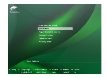
2. Select *Installation* on the boot screen, then press Enter. This loads the SUSE Linux Enterprise Server installation program and starts the installation in normal mode.
