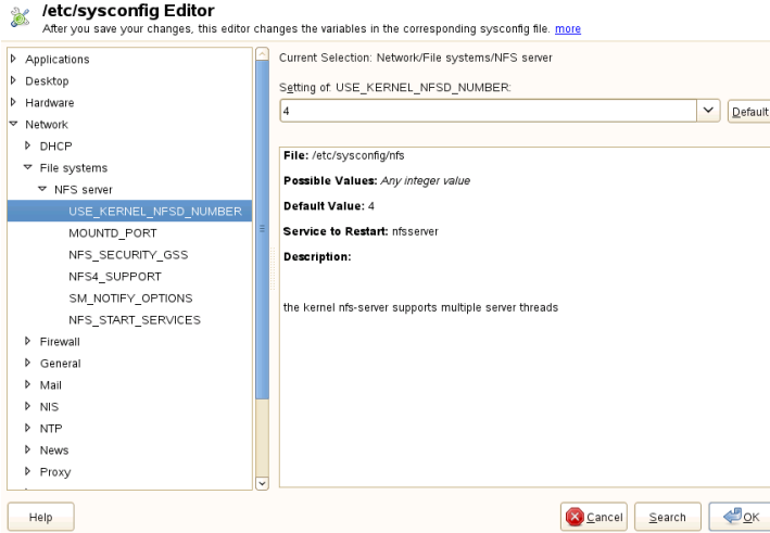
Figure 7.2 System Configuration Using the sysconfig Editor
